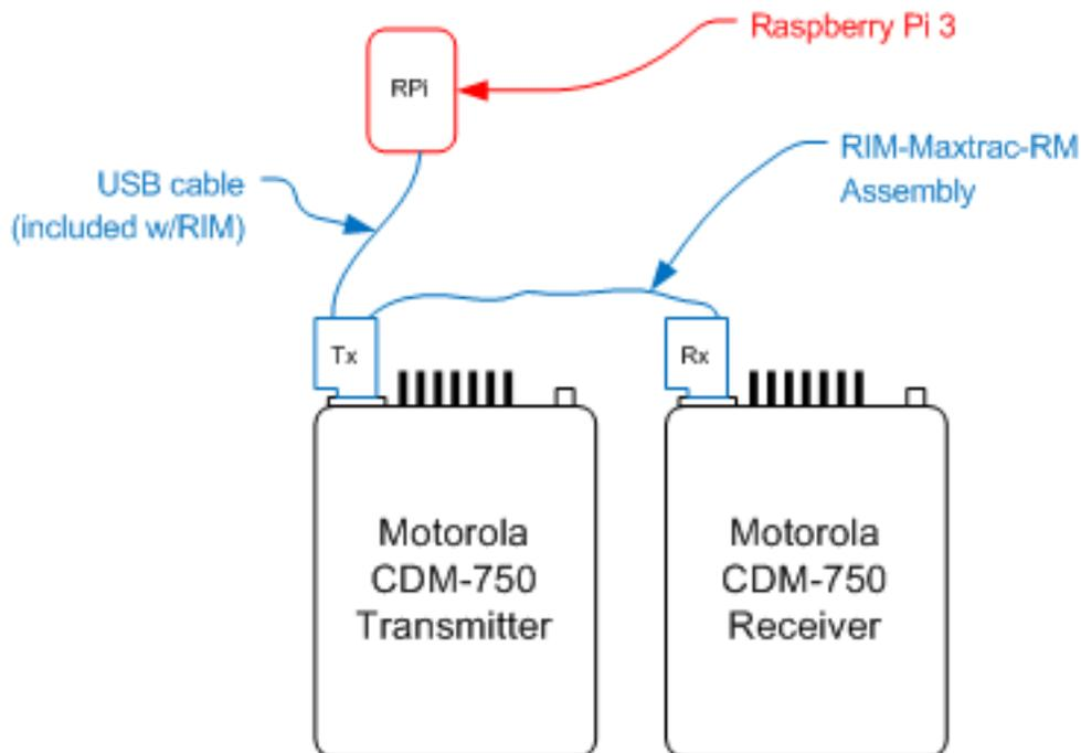
Add your duplexer, coax, antenna, and a power supply and this is all there is to it. You have a computer controlled repeater with voice ID and remote control that can link you anywhere in the world.
